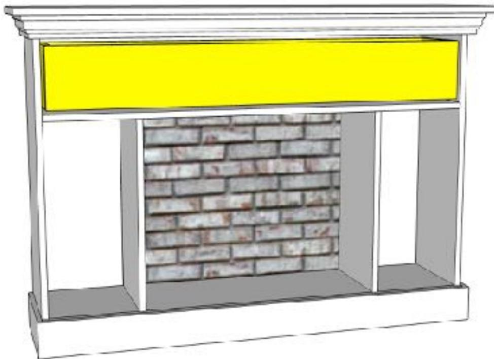
Install the drawer with 10" side mount drawer slides. Center the drawer slides on sides of the drawer opening on the fireplace as well as the sides of the drawer box. Attach with included screws.
