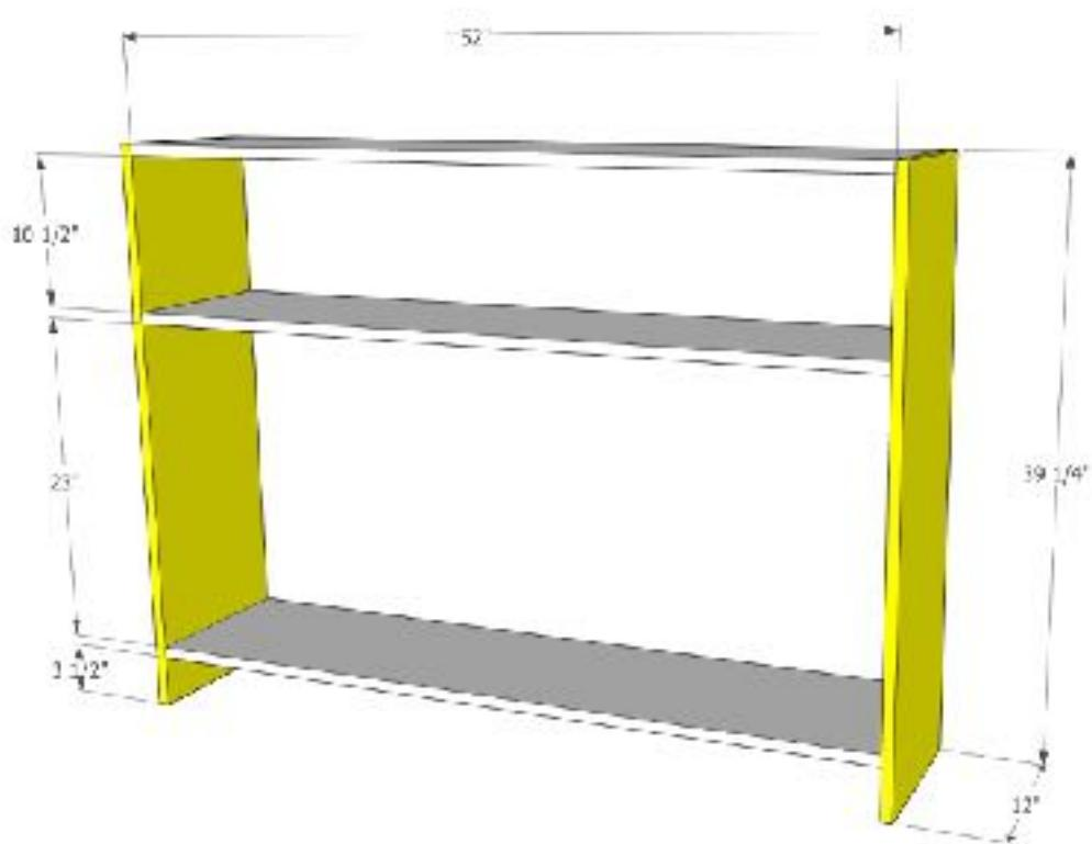
To build the carcass, drill  $3/4"$  pocket screws into each end of the top, middle, and bottom pieces. Apply veneer edge banding to all of the front edges of the carcass pieces. Trim the banding and sand the pieces smooth with 220 grit sandpaper. Assemble the carcass using wood glue and  $1\frac{1}{4}"$  pocket screws.
