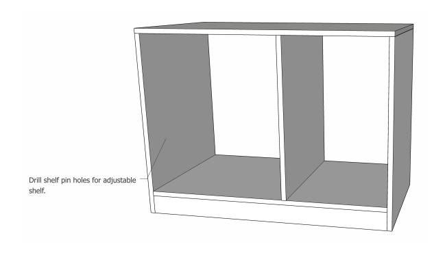
Using a shelf pin jig, drill the shelf pin holes on each side of the large opening for the adjustable shelf.
