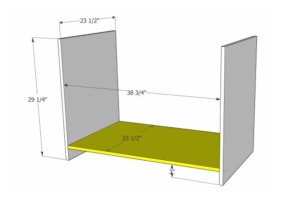
Drill 3/4" pocket holes into each end of the cabinet bottom. Also drill 3/4" pocket holes into the top edge of the cabinet sides. Mark 3" up on each of the cabinet side pieces. Place the cabinet bottom at the 3" mark. Attach with wood glue and 1 1/4" pocket screws.
