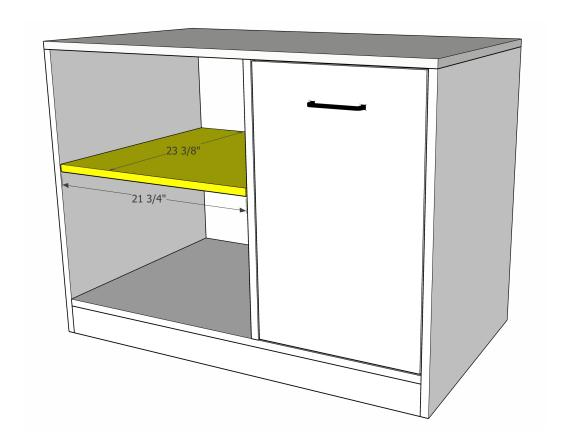
Finish the cabinet as desired with paint or stain. Install the drawer with 18" drawer slides. Install the adjustable shelf with shelf pins in coordinating color.
