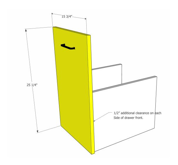
Attach the drawer front with a 1/2" overhang on each side, using wood glue and 1 1/4" pocket screws. Install the drawer pull.
