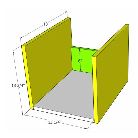
Drill 3/4" pocket holes into the front edge of the drawer sides, the front and sides of the drawer bottom, and the sides and bottom of the drawer back. Glue and attach the pieces together with 1 1/4" pocket screws.
