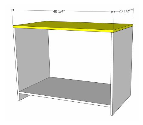
Attach the cabinet top using wood glue and 3/4" pocket screws. The ends of the top should be flush with the outside faces of the side panels.
