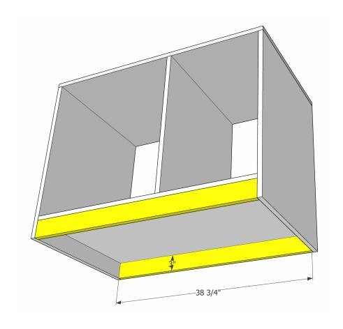
Drill 3/4" pocket holes into each end and one long side of the apron pieces. Attach to the bottom of the cabinet with wood glue and 1 1/4" pocket screws.
