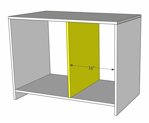
Drill 3/4" pocket holes into the top and bottom ends of the center divider. Mark 16" from one side (depending on which side you'd like the drawer), or cut a piece of scrap wood at 16" to act as a spacing block. Position the divider in place and attach with 1 1/4" pocket screws.
