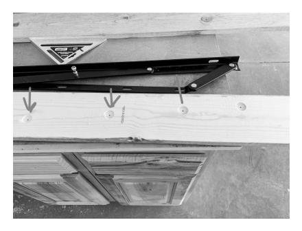
Flip the 1x6 over and, using a 1" forstner bit, drill 1/8" deep pilot holes. Use the 1/8' pilot holes as a centerpoint.
