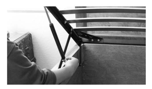
Attach the gas struts to the lift mechanism and bed frame.
