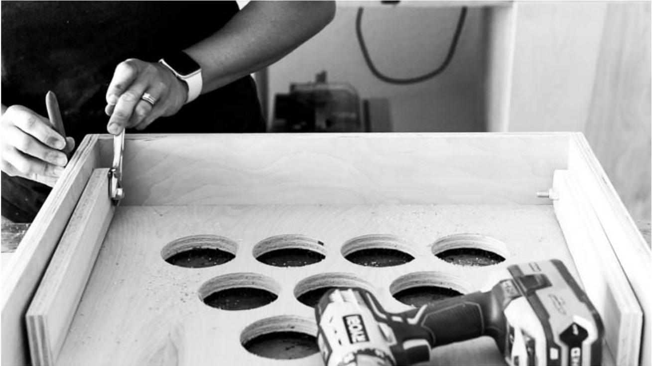
Use a 3/4" piece of wood as a block at the front edge of the game board frame. Place the leg against that block to set the location for the legs. Drill a 3/8" hole through each leg and through the side of the game board frame. Attach the legs with 2 1/2" carriage bolts and locking nuts, tightening them enough to hold the legs in position, but still allow for them to be folded back down into place when not in use.
