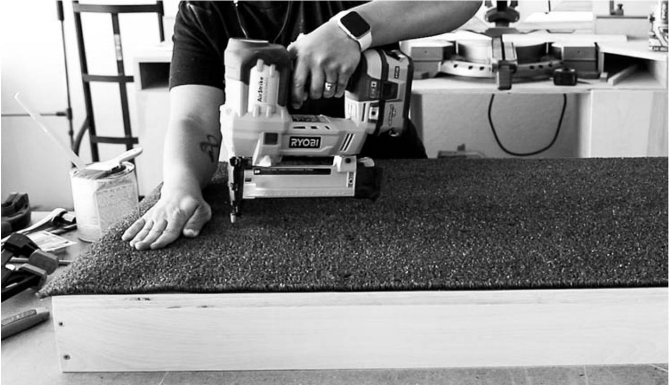
Cut the astro turf to size using a sharp razor knife. Apply a generous coat of contact cement onto the top of the game board with a paint brush. Align the grass over the game board and begin stapling it to the top starting at one edge and working your way down, smoothing out the grass as you go.
