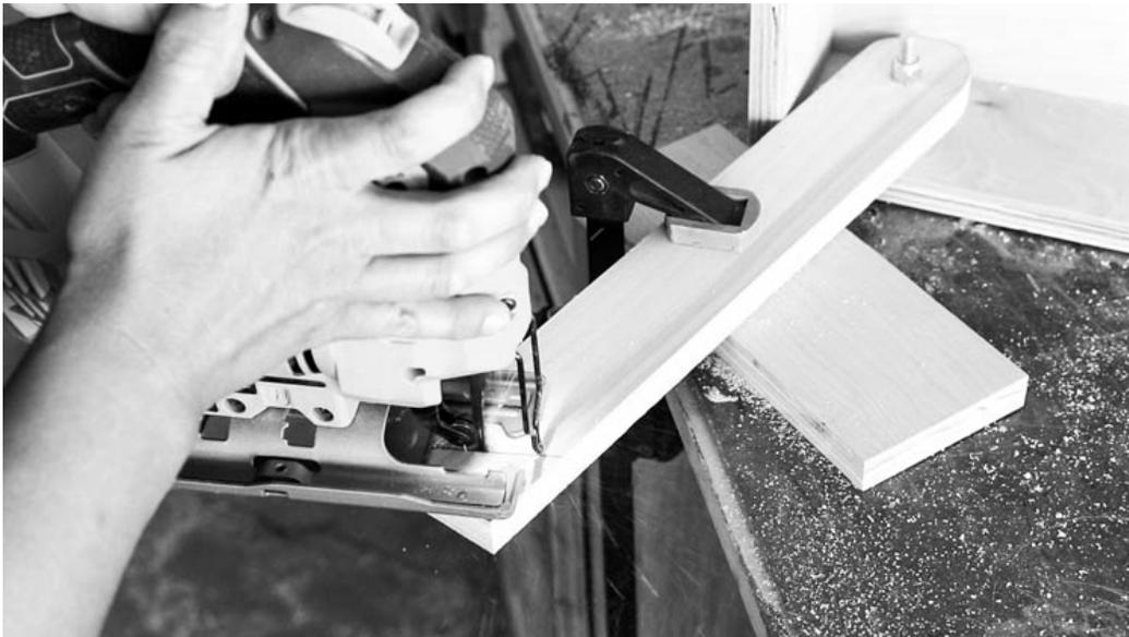
Stack two pieces of wood and place them next to the legs with the game board in upright position. Mark with a pencil the angle of the legs so that they will sit flush on the ground. Cut the ends of the legs with a jigsaw.
