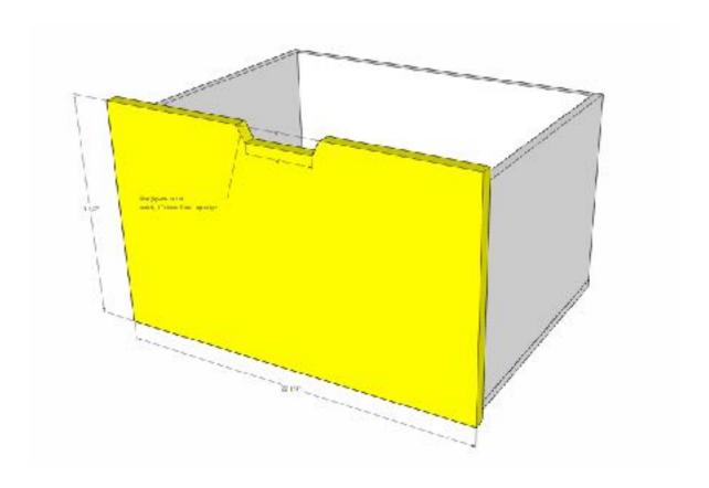
Measure and mark the notch for the drawer front based on the diagram above. Cut the notch with a jigsaw. Using wood glue and 1" pocket screws, attach the drawer front to the rest of the drawer box.
