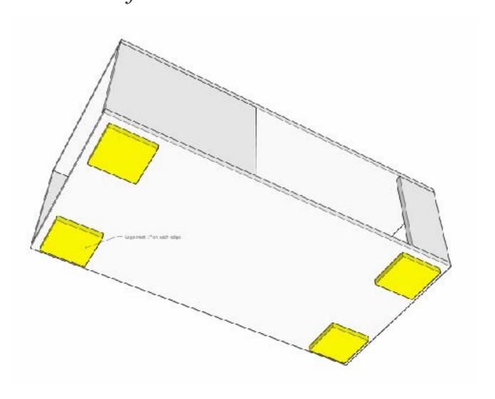
Measure and mark 1" in from the corners of the coffee table bottom. Apply wood glue to the feet and set in place so that they are 1" in from each corner edge. Nail in place with  $1\,1/4$ " brad nails.
