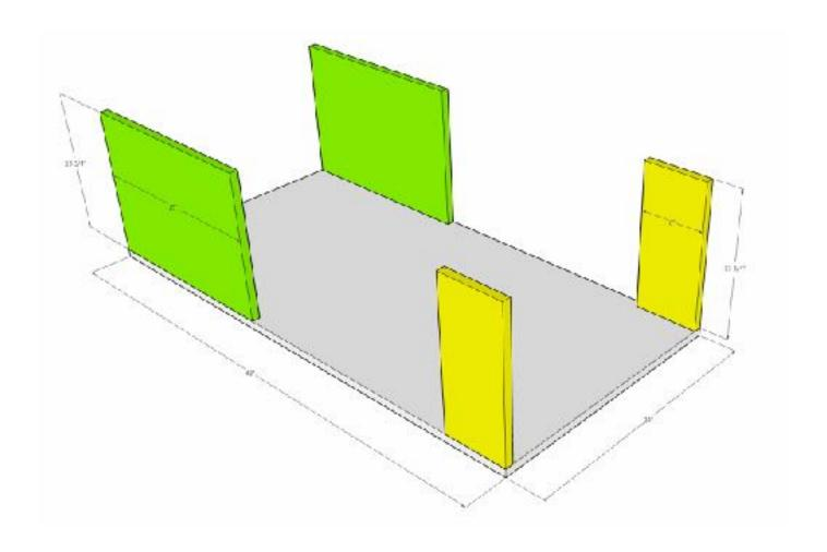
Drill 3/4" pocket holes into the upper and lower edges of the legs and side panels. Using wood glue and 11/4" pocket screws, attach the legs and side panels to the coffee table bottom.
