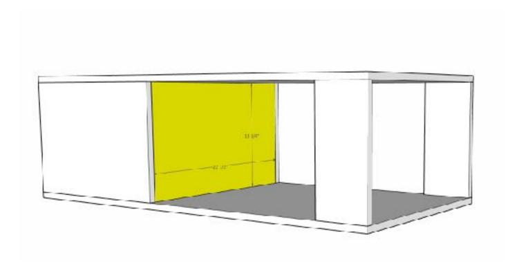
Drill 3/4" pocket holes into all four edges of the rear panel. Install flush with the edges of the side panels and clamp into place. Secure in place with 1 1/4" pocket screws.
