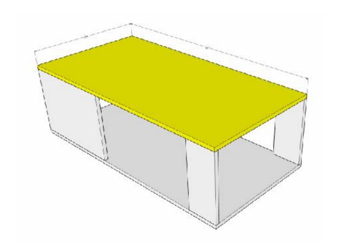
Using wood glue and 1 1/4" pocket screws attach the coffee table top to the legs and side panels, carefully clamping it into place and ensuring the panels and legs are square.
