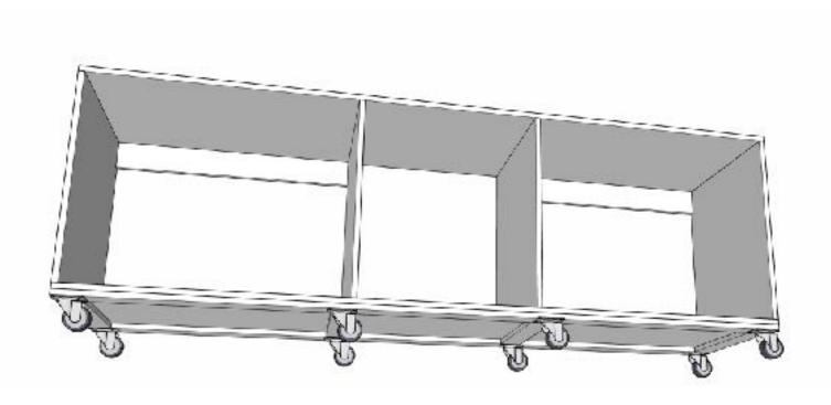
Attach the 3" swivel casters to the bottom of the miter saw bench using  $1\,1/4$ ", #12 wood screws with 1/4" finish washers. Attach the locking casters to the outside corners and the standard swivel casters to the center points.
