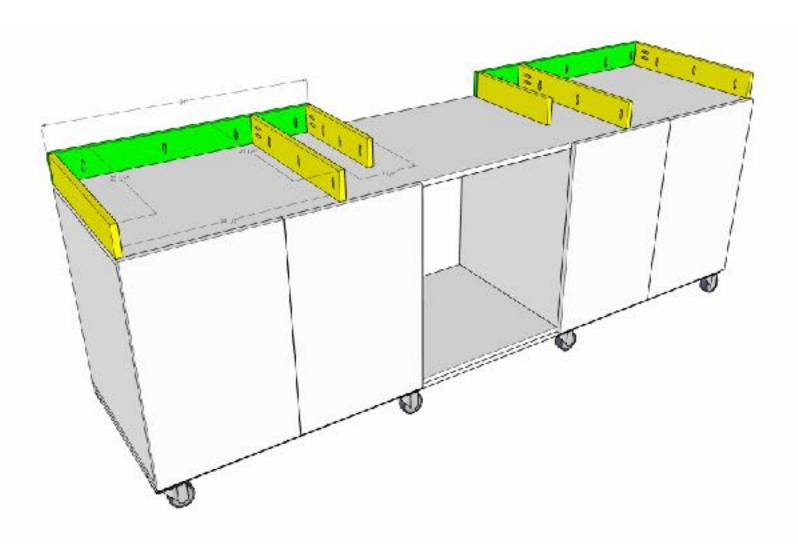
To build the frame for the table top, measure the height of the table top on your miter saw. Determine the height of the frame pieces based on the height of the miter saw table, and the thickness of the plywood being used for the table top.
