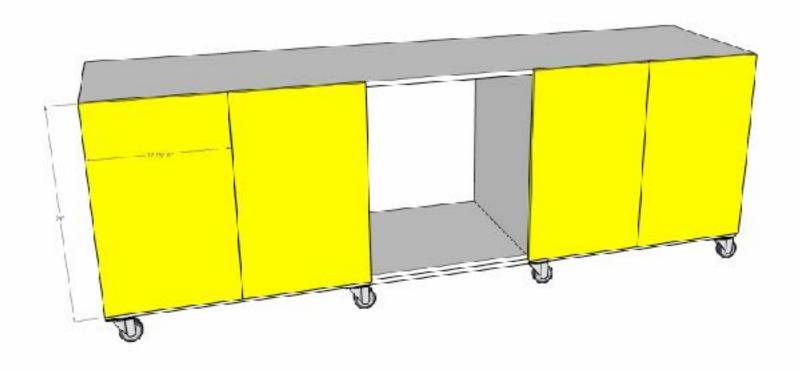
Install the cabinet doors. Measure 6" and mark from the top and bottom of the miter saw bench. Install the euro hinges at the marked locations. Attach the doors to the hinges, leaving a 1/8" gap between the doors.
