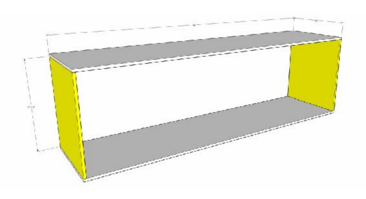
Drill 3/4" pocket holes into the upper and lower edges of the side pieces that make up the main carcass of the miter saw bench. Glue and clamp into place. Attach to the top and bottom pieces with 1 1/4" pocket screws.
