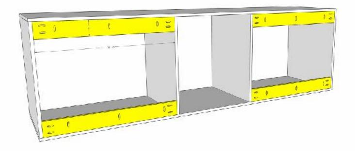
Drill 3/4" pocket holes into the ends and one edge of each of the rear stretchers. These will provide stability to the miter saw bench. Glue and clamp into place, attaching with  $1\,1/4$ " pocket screws.
