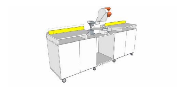
Position your miter saw centered in between the table top risers. Make sure that the fence of the miter saw is square to the sides of the table top. Drill 3/4" pocket holes into the fence peices. Square up the plywood fence pieces to the fence on the miter saw and secure them in place with clamps and scrap wood (see accompanying video for this step). Glue and attach in place with 1 1/4" pocket screws.
