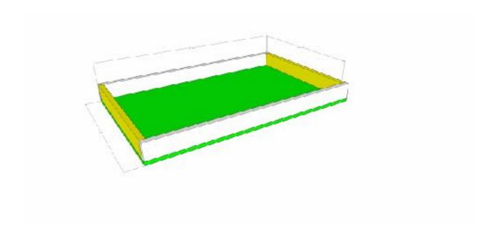
To build the pull out shelves, drill 3/4" pocket holes into the 20 1/2" side pieces. Glue and clamp the box together and attach the sides with 1 1/4" pocket screws. Attach the shelf bottom with wood glue and 1 1/4" wood screws.
