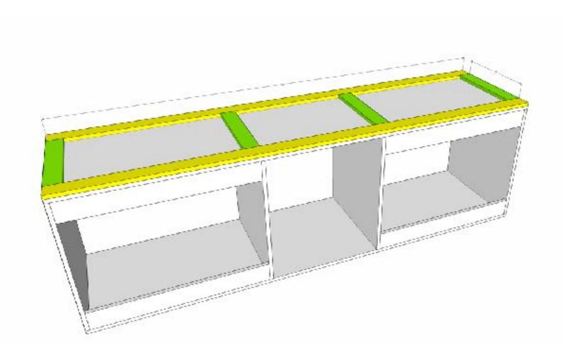
Cut the bottom support frame pieces to size. Attach the 8' pieces first, then attach the 18" pieces using wood glue and 1 1/4" wood screws.
