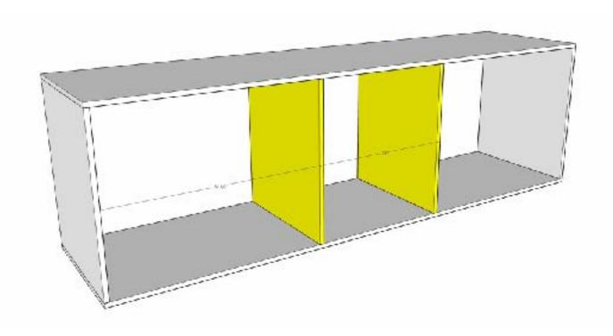
Measure and mark the locations for the center divider placement. Drill 3/4" pocket holes into the upper and lower edges of the center dividers. Glue and clamp into place following the spacing diagram above and attach with 1 1/4" pocket screws.
