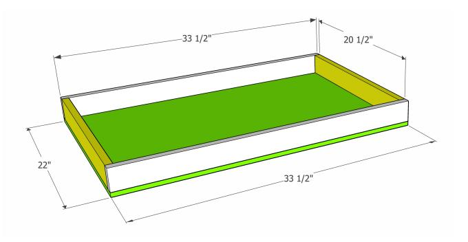
To build the pull out shelves, drill 3/4" pocket holes into the 20 1/2" side pieces. Glue and clamp the box together and attach the sides with 1 1/4" pocket screws. Attach the shelf bottom with wood glue and 1 1/4" wood screws.
