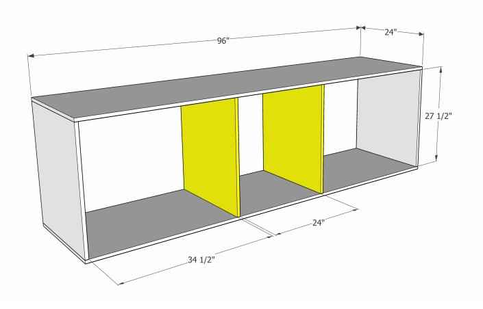
Measure and mark the locations for the center divider placement. Drill 3/4" pocket holes into the upper and lower edges of the center dividers. Glue and clamp into place following the spacing diagram above and attach with 1 1/4" pocket screws.
