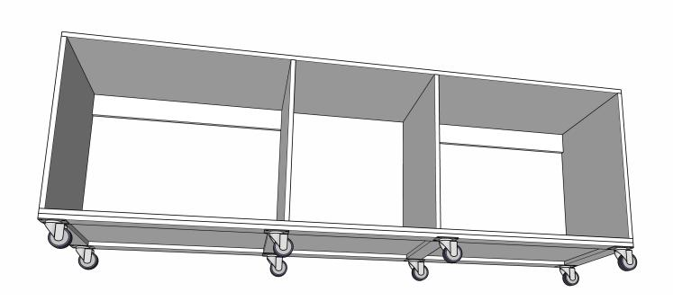
Attach the 3" swivel casters to the bottom of the miter saw bench using  $1\,1/4$ ", #12 wood screws with 1/4" finish washers. Attach the locking casters to the outside corners and the standard swivel casters to the center points.
