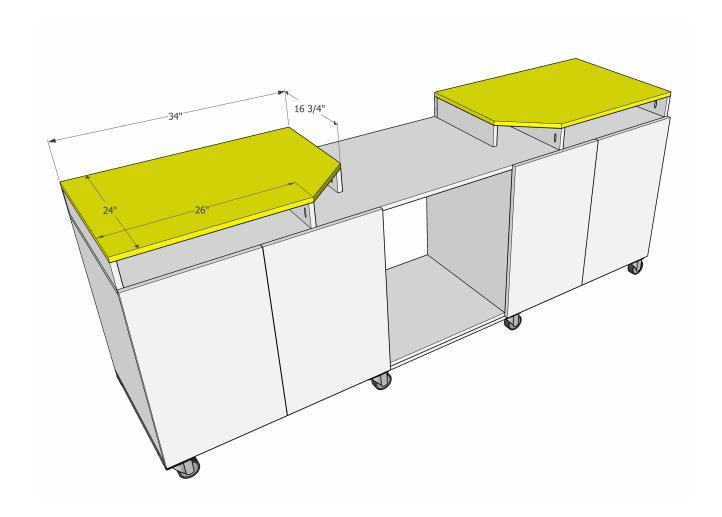
Measure and mark the table tops where the corners will be cut off to accommodate the swing of the miter saw base. Cut the corners off with a jigsaw. Attach to the table top frame using wood glue and  $1\,1/4$ " wood screws.
