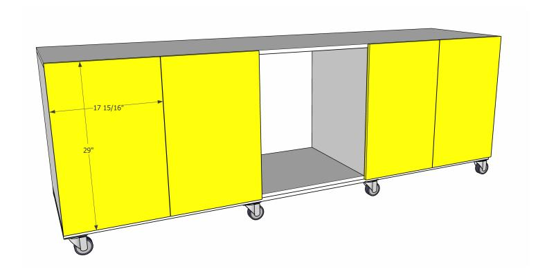
Install the cabinet doors. Measure 6" and mark from the top and bottom of the miter saw bench. Install the euro hinges at the marked locations. Attach the doors to the hinges, leaving a 1/8" gap between the doors.
