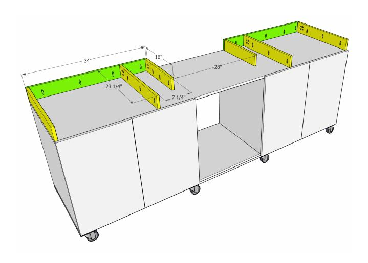
To build the frame for the table top, measure the height of the table top on your miter saw. Determine the height of the frame pieces based on the height of the miter saw table, and the thickness of the plywood being used for the table top.
