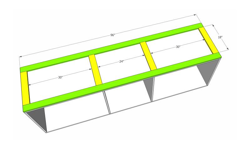
Cut the bottom support frame pieces to size. Attach the 8' pieces first, then attach the 18" pieces using wood glue and  $1\,1/4$ " wood screws.
