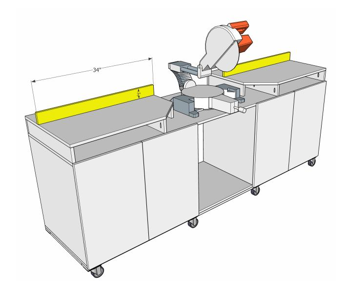
Position your miter saw centered in between the table top risers. Make sure that the fence of the miter saw is square to the sides of the table top. Drill 3/4" pocket holes into the fence peices. Square up the plywood fence pieces to the fence on the miter saw and secure them in place with clamps and scrap wood (see accompanying video for this step). Glue and attach in place with 1 1/4" pocket screws.
