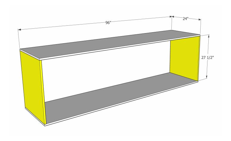
Drill 3/4" pocket holes into the upper and lower edges of the side pieces that make up the main carcass of the miter saw bench. Glue and clamp into place. Attach to the top and bottom pieces with  $1 \frac{1}{4}$ " pocket screws.
